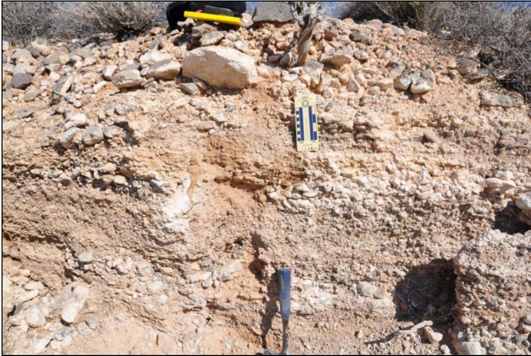
Figure 2-46: Gully cut bank revealing the gravelly calcic soil profile of unit Qa1.
