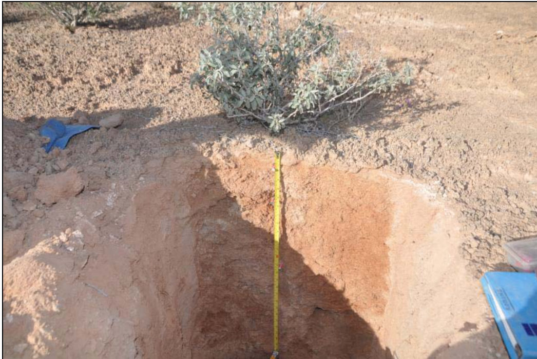
Figure 2-32: Soil profile excavation in unit Qea below a buckwheat plant.
